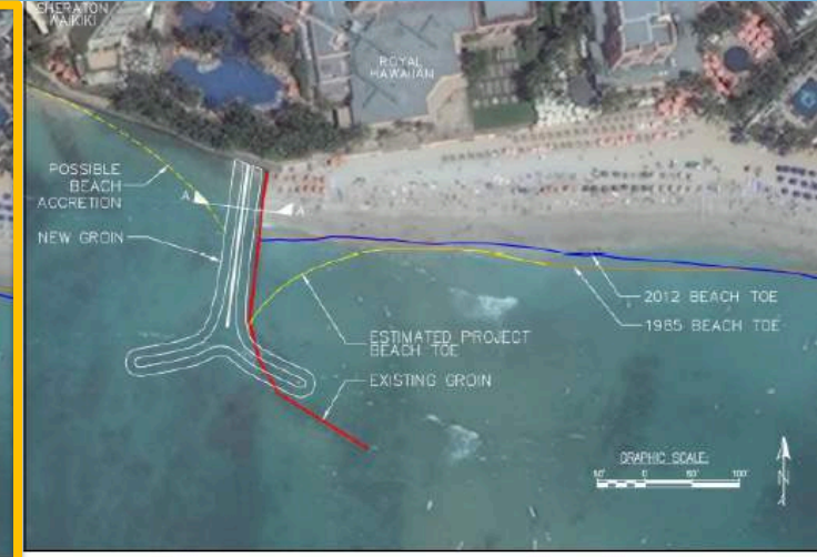
Figure 2-3 Plan view of 280-foot long groin
