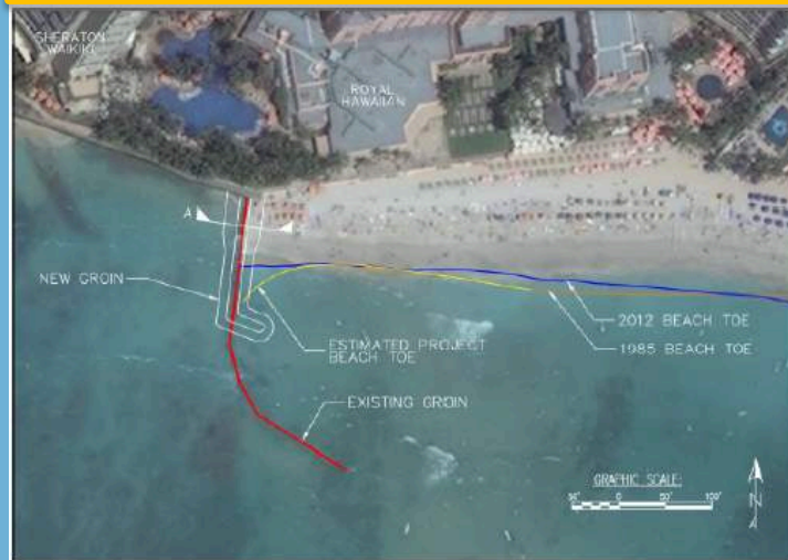
Figure 2-4 Adaptive Reuse groin plan view
