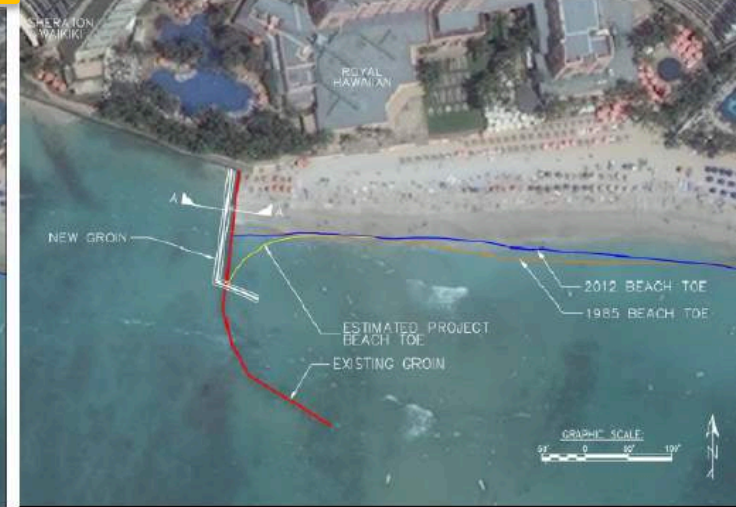
Figure 2-6 Concrete wall groin plan view
