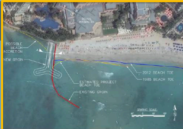
Figure 2-1 Plan view of proposed 180-foot long groin
