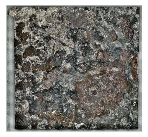
Figure 155. A screenshot of the 3D digital image of a specimen excised from Coupon 3 labeled as 3-1, after CO<sub>2</sub> blast cleaning
