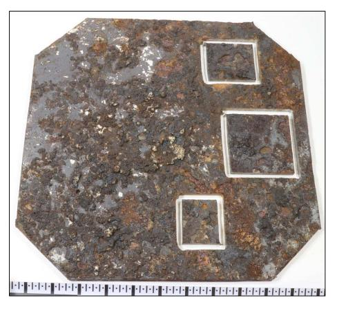
Figure 139. An image of the interior surface of Coupon 7 after CO<sub>2</sub> blast cleaning.
