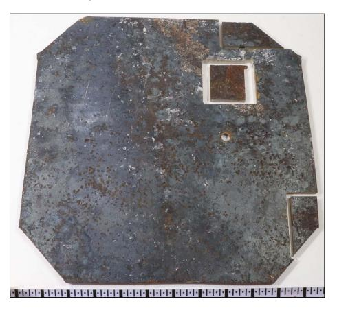
Figure 137. An image of the interior surface of Coupon 6 after CO<sub>2</sub> blast cleaning.
