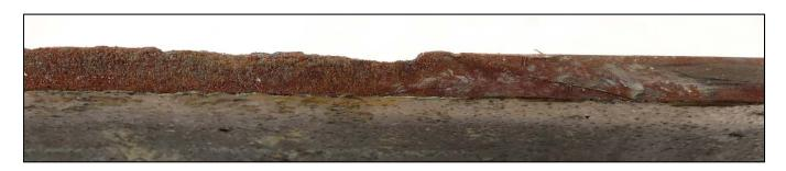
**Figure 27.** An image of a representative edge of Coupon A1 in the as-received condition.
