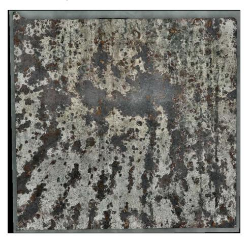
**Figure 149.** A screenshot of the 3D digital image of a specimen excised from Coupon 1 labeled as 1-1, after CO<sub>2</sub> blast cleaning
