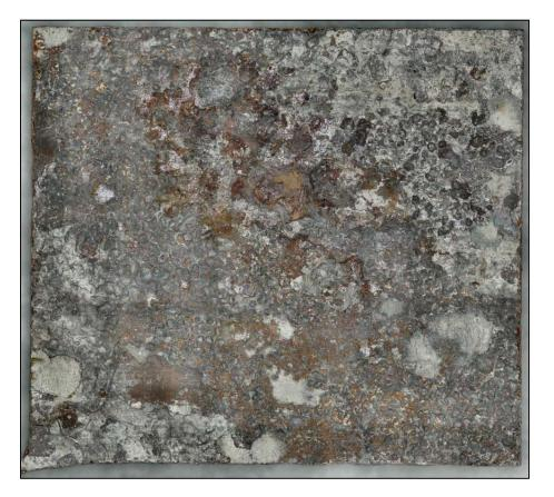
**Figure 175.** A screenshot of the 3D digital image of a specimen excised from Coupon A-1 labeled as A1-2, after CO<sub>2</sub> blast cleaning
