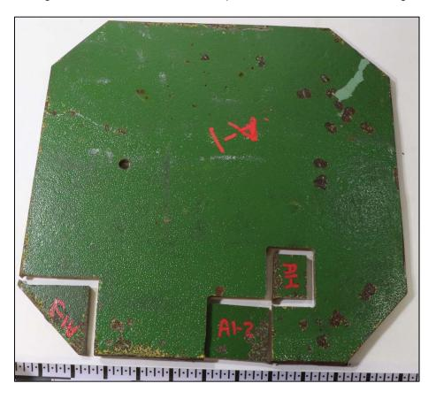
Figure 146. An image of the exterior surface of Coupon A1 after CO<sub>2</sub> blast cleaning.
