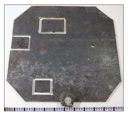
Figure 135. An image of the interior surface of Coupon 5 after CO<sub>2</sub> blast cleaning.
