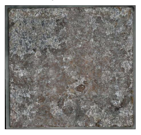
**Figure 170.** A screenshot of the 3D digital image of a specimen excised from Coupon 8 labeled as 8-3, after CO<sub>2</sub> blast cleaning
