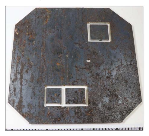
Figure 129. An image of the interior surface of Coupon 1 after CO<sub>2</sub> blast cleaning.
