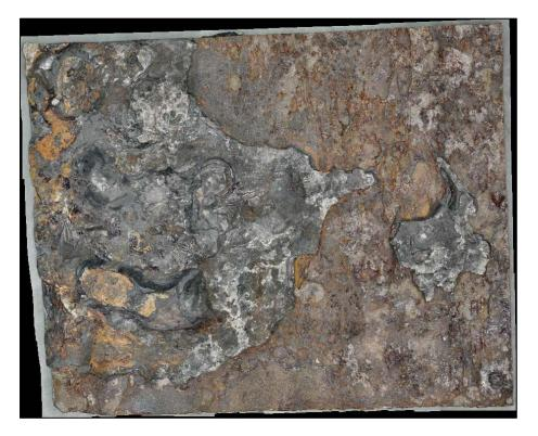
**Figure 157.** A screenshot of the 3D digital image of a specimen excised from Coupon 3 labeled as 3-3, after CO<sub>2</sub> blast cleaning
