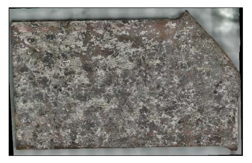
**Figure 168.** A screenshot of the 3D digital image of a specimen excised from Coupon 8 labeled as 8-1, after CO<sub>2</sub> blast cleaning
