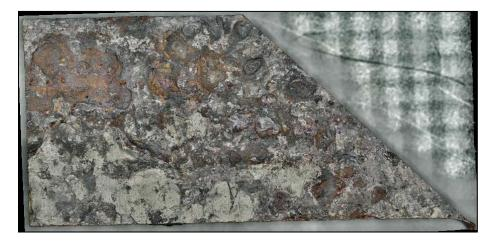
**Figure 162.** A screenshot of the 3D digital image of a specimen excised from Coupon 6 labeled as 6-2, after CO<sub>2</sub> blast cleaning
