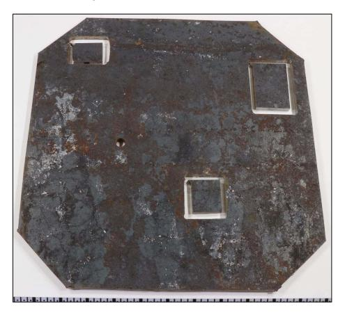
Figure 147. An image of the interior surface of Coupon A2 after CO<sub>2</sub> blast cleaning.
