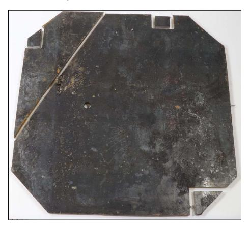
**Figure 143.** An image of the interior surface of Coupon 10 after CO<sub>2</sub> blast cleaning.
