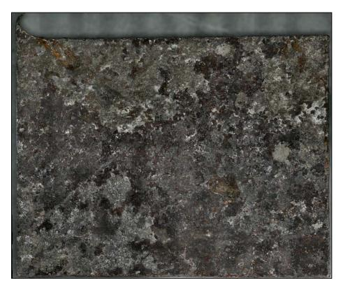
**Figure 160.** A screenshot of the 3D digital image of a specimen excised from Coupon 5 labeled as 5-3, after CO<sub>2</sub> blast cleaning
