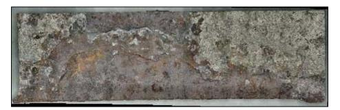
**Figure 154.** A screenshot of the 3D digital image of a specimen excised from Coupon 2 labeled as 2-3, after CO<sub>2</sub> blast cleaning
