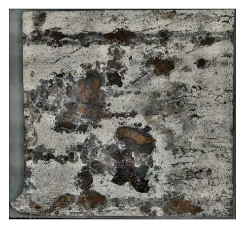
**Figure 150.** A screenshot of the 3D digital image of a specimen excised from Coupon 1 labeled as 1-2, after CO<sub>2</sub> blast cleaning
