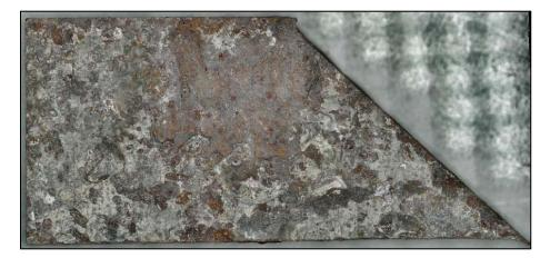
**Figure 163.** A screenshot of the 3D digital image of a specimen excised from Coupon 6 labeled as 6-3, after CO<sub>2</sub> blast cleaning
