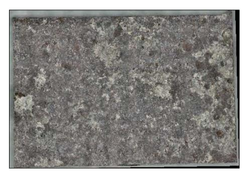
**Figure 178.** A screenshot of the 3D digital image of a specimen excised from Coupon A-2 labeled as A2-2, after CO<sub>2</sub> blast cleaning
