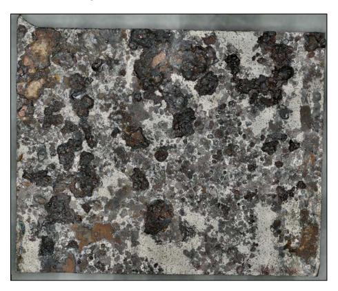
**Figure 151.** A screenshot of the 3D digital image of a specimen excised from Coupon 1 labeled as 1-3, after CO<sub>2</sub> blast cleaning
