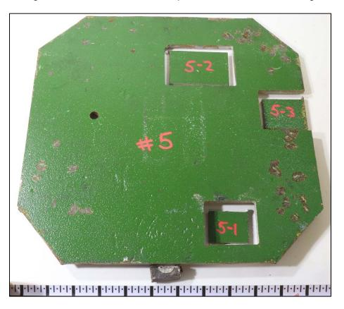
Figure 136. An image of the exterior surface of Coupon 5 after CO<sub>2</sub> blast cleaning.
