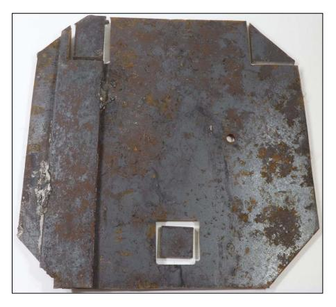
Figure 141. An image of the interior surface of Coupon 8 after CO<sub>2</sub> blast cleaning.
