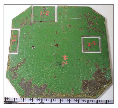
Figure 132. An image of the exterior surface of Coupon 2 after CO<sub>2</sub> blast cleaning.
