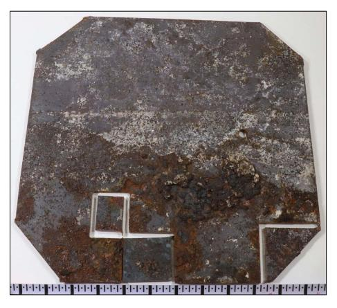
**Figure 145.** An image of the interior surface of Coupon A1 after CO<sub>2</sub> blast cleaning.
