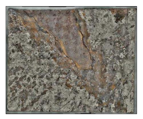
**Figure 152.** A screenshot of the 3D digital image of a specimen excised from Coupon 2 labeled as 2-1, after CO<sub>2</sub> blast cleaning
