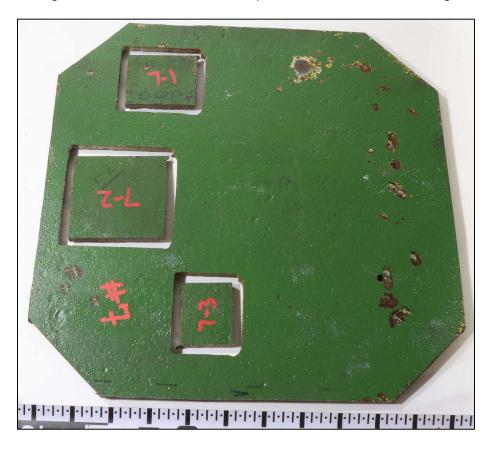
Figure 140. An image of the exterior surface of Coupon 7 after CO<sub>2</sub> blast cleaning.
