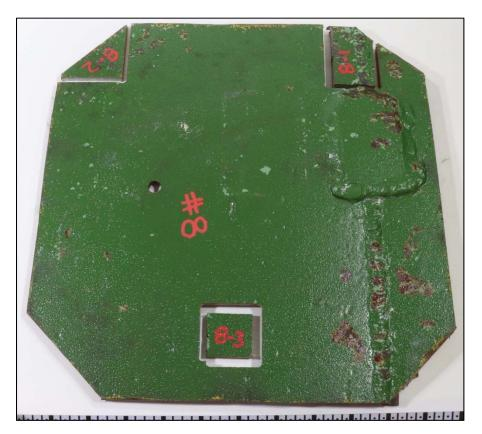
Figure 142. An image of the exterior surface of Coupon 8 after CO<sub>2</sub> blast cleaning.
