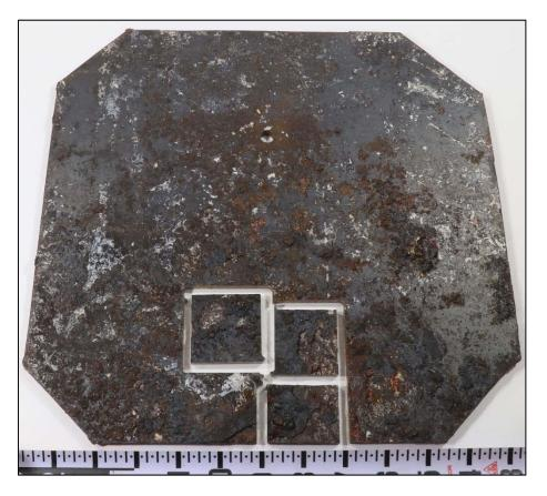
**Figure 133.** An image of the interior surface of Coupon 3 after CO<sub>2</sub> blast cleaning.
