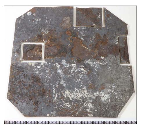
Figure 131. An image of the interior surface of Coupon 2 after CO<sub>2</sub> blast cleaning.
