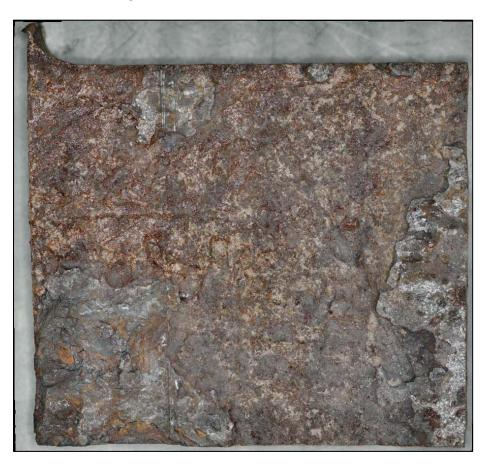
**Figure 161.** A screenshot of the 3D digital image of a specimen excised from Coupon 6 labeled as 6-1, after CO<sub>2</sub> blast cleaning
