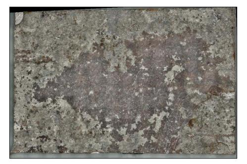
**Figure 159.** A screenshot of the 3D digital image of a specimen excised from Coupon 5 labeled as 5-2, after CO<sub>2</sub> blast cleaning
