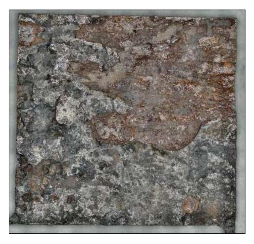
**Figure 156.** A screenshot of the 3D digital image of a specimen excised from Coupon 3 labeled as 3-2, after CO<sub>2</sub> blast cleaning
