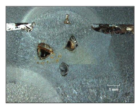
**Figure 212.** The right-hand feature in Figure 210 is shown at higher magnification. The weld indications appeared to be porosity.
