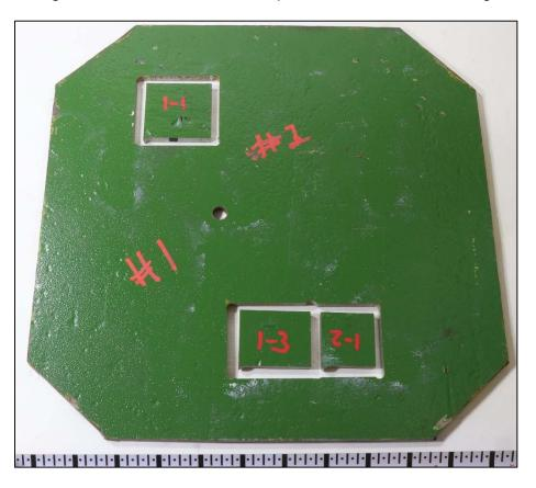
Figure 130. An image of the exterior surface of Coupon 1 after CO<sub>2</sub> blast cleaning.
