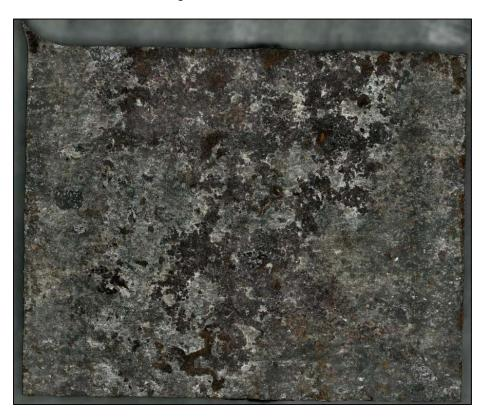
**Figure 158.** A screenshot of the 3D digital image of a specimen excised from Coupon 5 labeled as 5-1, after CO<sub>2</sub> blast cleaning
