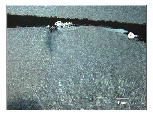
**Figure 209.** The location identified in the previous figure is shown at higher magnification. The weld indication (arrow) appeared to be an area of incomplete fusion.
