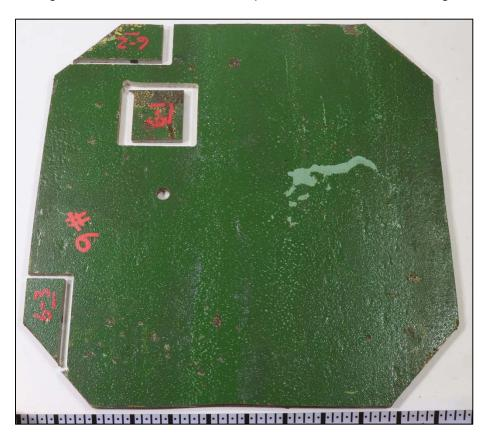
Figure 138. An image of the exterior surface of Coupon 6 after CO<sub>2</sub> blast cleaning.
