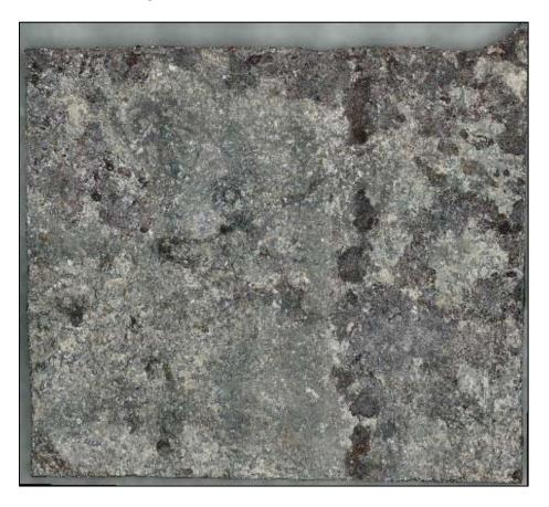
**Figure 177.** A screenshot of the 3D digital image of a specimen excised from Coupon A-2 labeled as A2-1, after CO<sub>2</sub> blast cleaning
