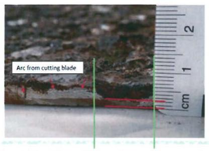
Figure 1: Edge of Coupon #7. Image from non-Navy source alleging the thickness of the remaining steel at the location shown between the two red lines was no more than 2 millimeters, less than the Navy's predictions. The label "Arc from cutting blade" was added by the laboratory to help demonstrate that all 3 photos shown are of the same location of coupon #7.
