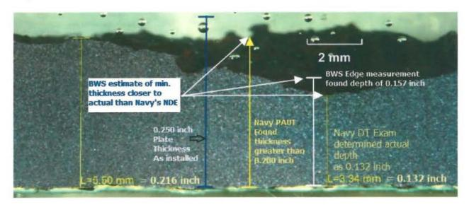
In this specific instance, the BWS edge estimate, based only on the crude measurements allowed by the Navy, were significantly closer to the actual plate minimum thickness. For Coupon #7 it is true that "the corrosion was far worse than the Navy expected."
