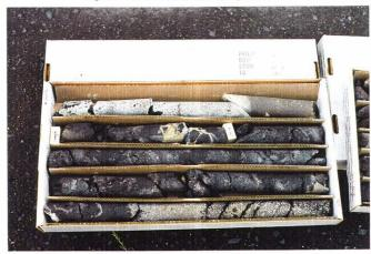
Figure 4-8 Petroleum Stained Core - B16C, 60' to 69'
