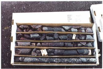
Figure 4-7 Petroleum Stained Core - B16C, 49' to 60
