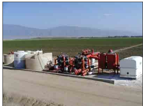
Chemigation is the addition of fertilizers or pesticides directly to irrigation water. Source: http://groups.ucanr.org/kernag/Chemigation/
