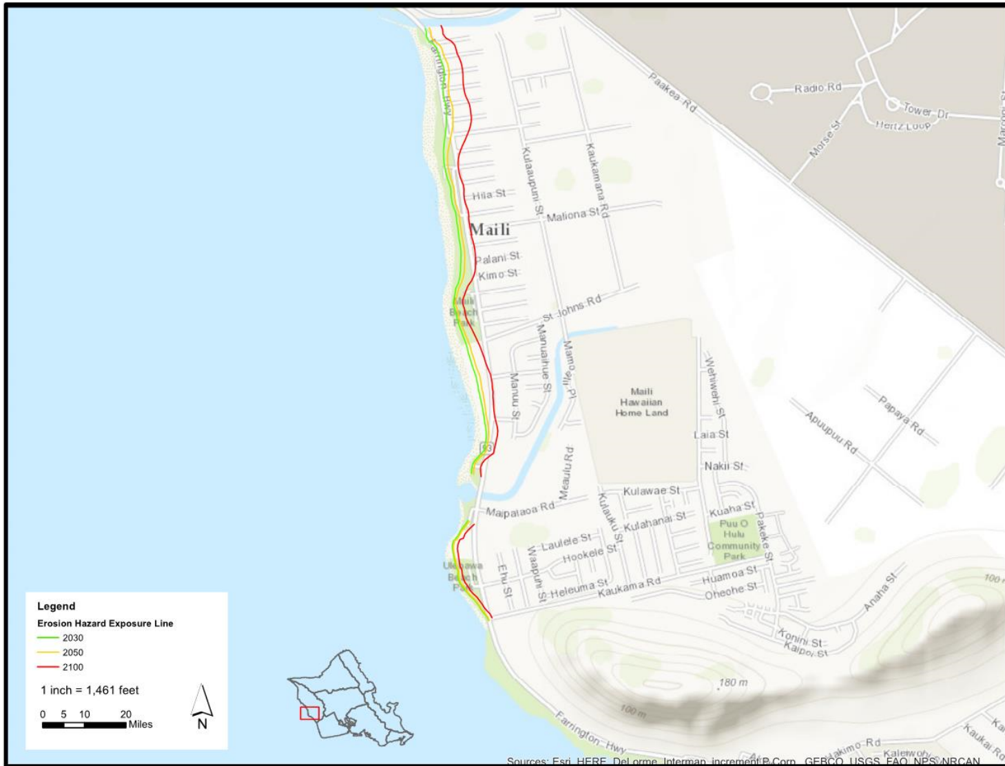
Figure A-3. Erosion Hazard Exposure with Sea Level Rise in 2030, 2050, and 2100 in Maili.
