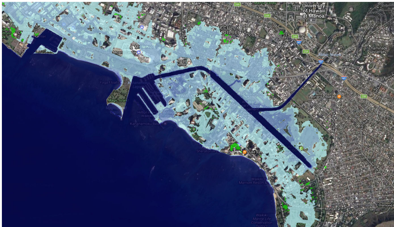
Figure 4-11. Groundwater Inundation and Marine Inundation in Waikiki with 5 ft of Sea Level Rise. Groundwater inundation shown in green. Marine inundation shown in blue. Source: NOAA 2018.
