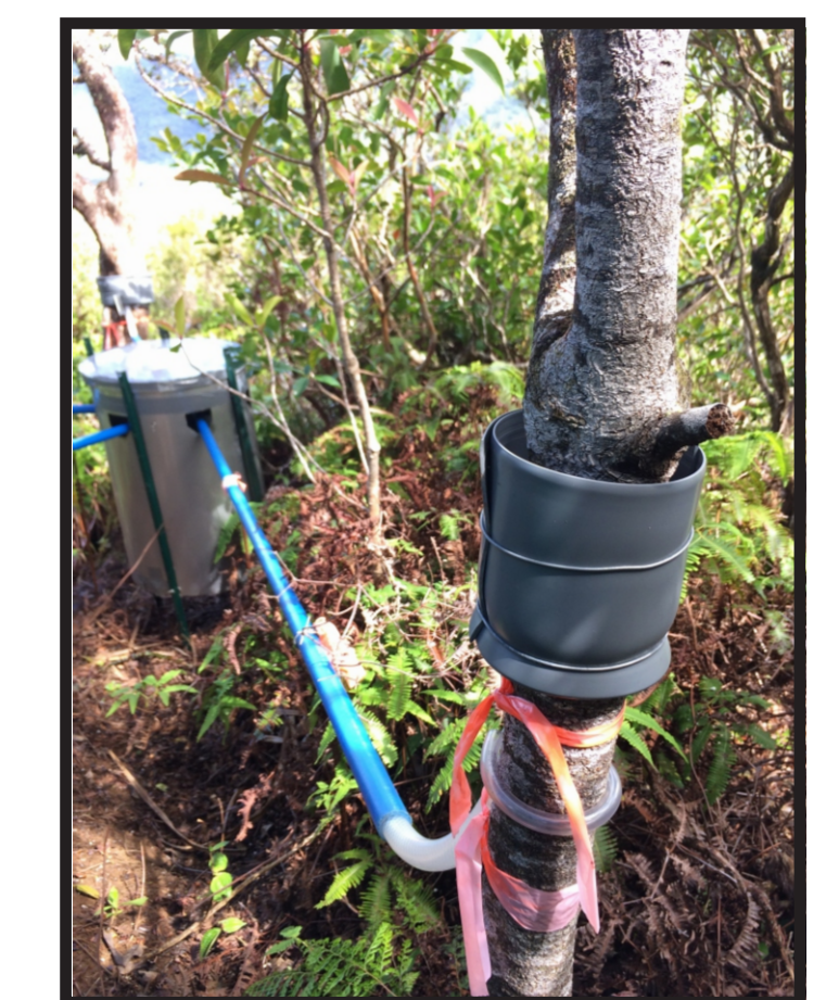
Stemflow Equipment: Stemflow collectors connected to a fabricated tipping bucket (150 mL / tip) rain gauge were used for each test plot. Trees selected for stemflow data collection represented the range of typical species, diameter and height found commonly on the test plots. Stemflow collectors were supported through lengths of 7/8-inch diameter poly tubing protected in 1-inch diameter HDPE pipe, leading toward the rain gauge, nested in a stainless steel can, levelled and anchored.
