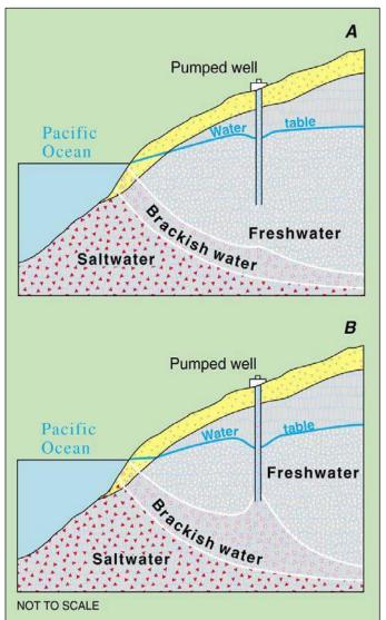
Saltwater intrusion is a potential problem near the coast. (**A**) Diagram of a well completed in a volcanic-rock aquifer in which withdrawal is small. Only limited saltwater intrusion has taken place. (**B**) Diagram of the same well under conditions of large ground-water withdrawal. Pumping has lowered the water table and caused the freshwater lens to thin. Brackish water has reached the well.
