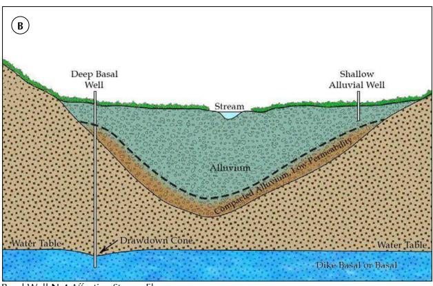
Basal Well **Not** Affecting Stream Flow Alluvial Well Potentially Affecting Stream Flow
