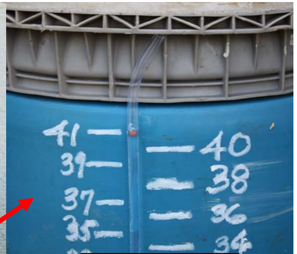
Water level gauge made out of plastic tubing and small piece of plastic
