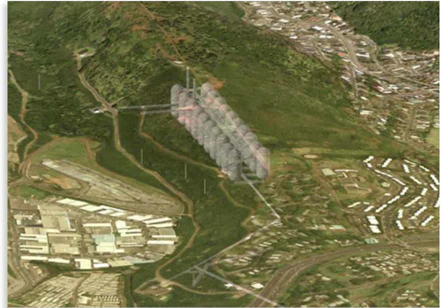
The location of underground tanks are illustrated in this aerial photo of the U.S. Navy's Red Hill Bulk Fuel Storage Facility in Hālawā. Ref. Red Hill Bulk Fuel Storage Facility Final Technical Report, 2007, Fig. 1-3, p. 1-15.
